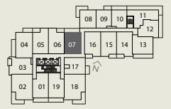
5TH - 7TH FLOORS 9'-0" CEILINGS UNITS 1-19 ON 5TH & 6TH FLOORS. 9'-0" CEILINGS UNITS 8-16 ON 7TH FLOOR. 9'-10" CEILINGS UNITS 1-7 & 17-19 ON 7TH FLOOR.
